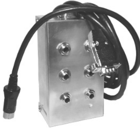
Figure 26: Conversion Cable and "Break-out" Box
